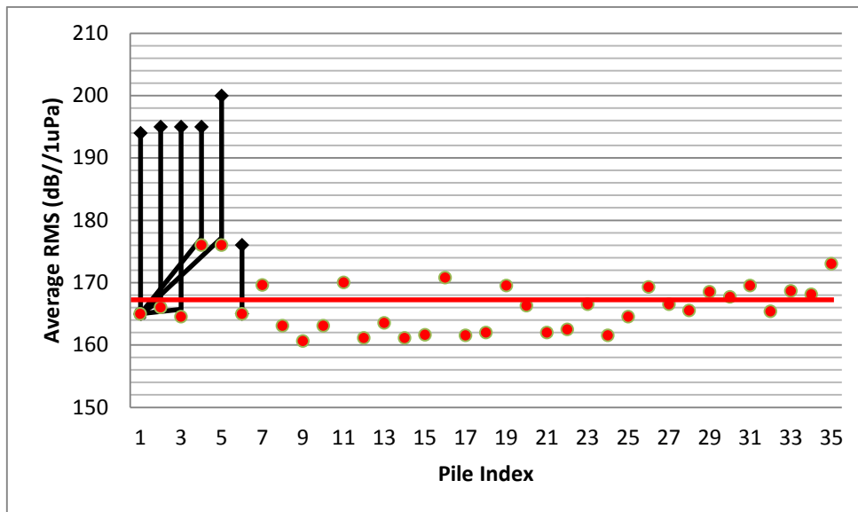
Figure B-24. 30-inch RMS Vibratory Measurements
